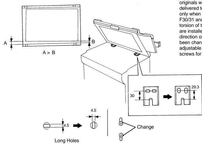
originals were sometimes skewed when delivered to the exposure glass. This happened only when this ARDF unit was installed on the F30/31 and F33/34 unit. This is due to the torsion of the upper cover on which the hinges are installed. To correct this, position and direction of the long hole of the right hinge has been changed. The skewed original is adjustable by changing the position of the screws for the right hinge.
